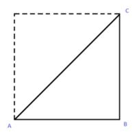
Triangle ABC shown above is a special kind of right angled triangle. Side AB is equal in length to side BC. This is the kind of triangle you get when you cut a square diagonally. The angles are 45°, 90°, 45°.
