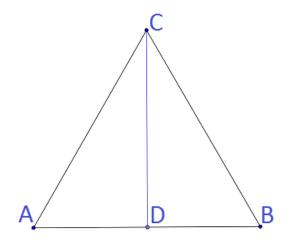
The triangle ABC is an equilateral triangle. All its sides are the same length. The blue line from point C to point D divides this equilateral triangle into two triangles that are exact mirror images of each other. Because angle ADC and angle BDC are equal and add up to 180 degrees, they are each 90 degrees.
